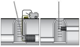
ALWAYS BLOCK PLUGS WHEN CONDUCTING AIR TESTS.
