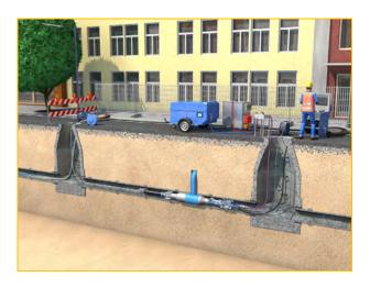
In this system, a flexible tube (liner) made of a corrosion-proof polyester fibre, coated outside, is wetted inside with a reaction resin (two component epoxy).
