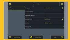
Annotate footage with details like manhole numbers, survey direction, distance and operator. Combine data, video and still images into complete surveys.
