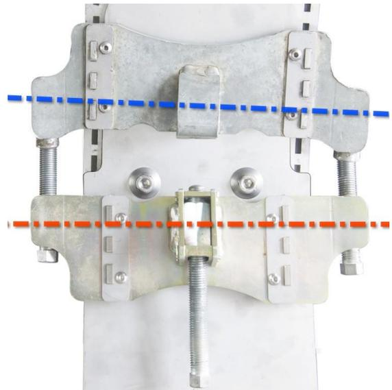
**Tightening the locking screws**
