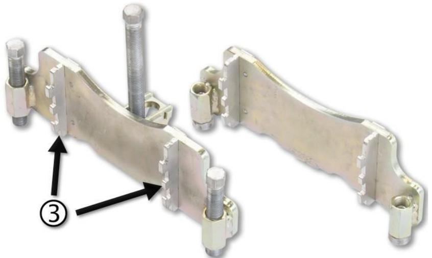
Depending on the pipe diameter, the retaining lugs (3) on the installation tool may have to be changed. These parts are supplied with the tools.
