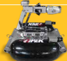
FLOAT Turn your RX130 into a floating inspection tool with tether points at front and rear.
